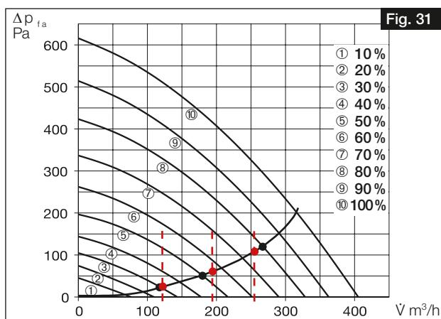
2. The approximate fan powers to be set (in %) can be read from the ventilation profiles at the points of intersection of the flow rates and the system characteristic curve. Enter these in the corresponding ventilation profile via the easy-Controls software or the control element KWL-BE Touch (cf. Fig. 31 and Fig. 32).
