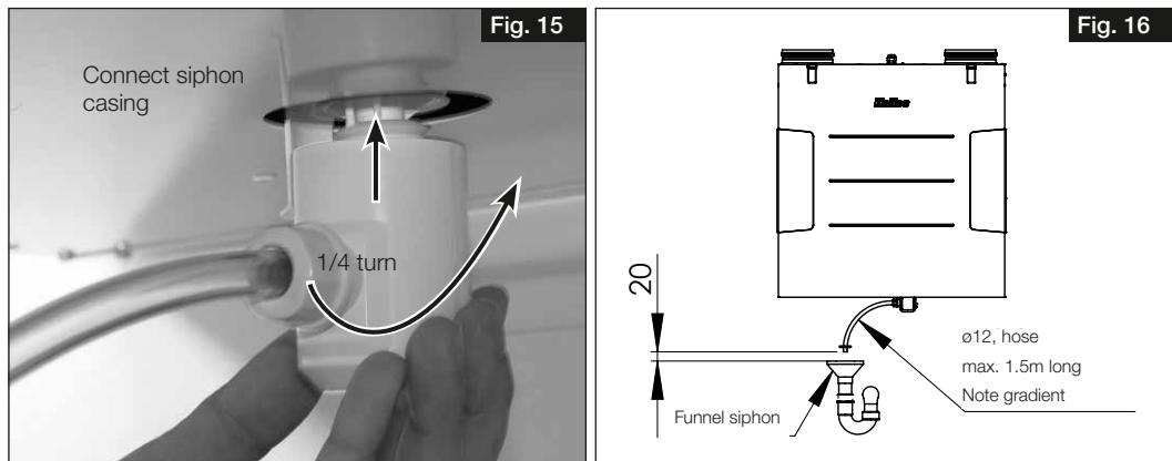
6. Connect condensate hose (length max. 1.5 m) to the building drainage system (see Fig. 17).
