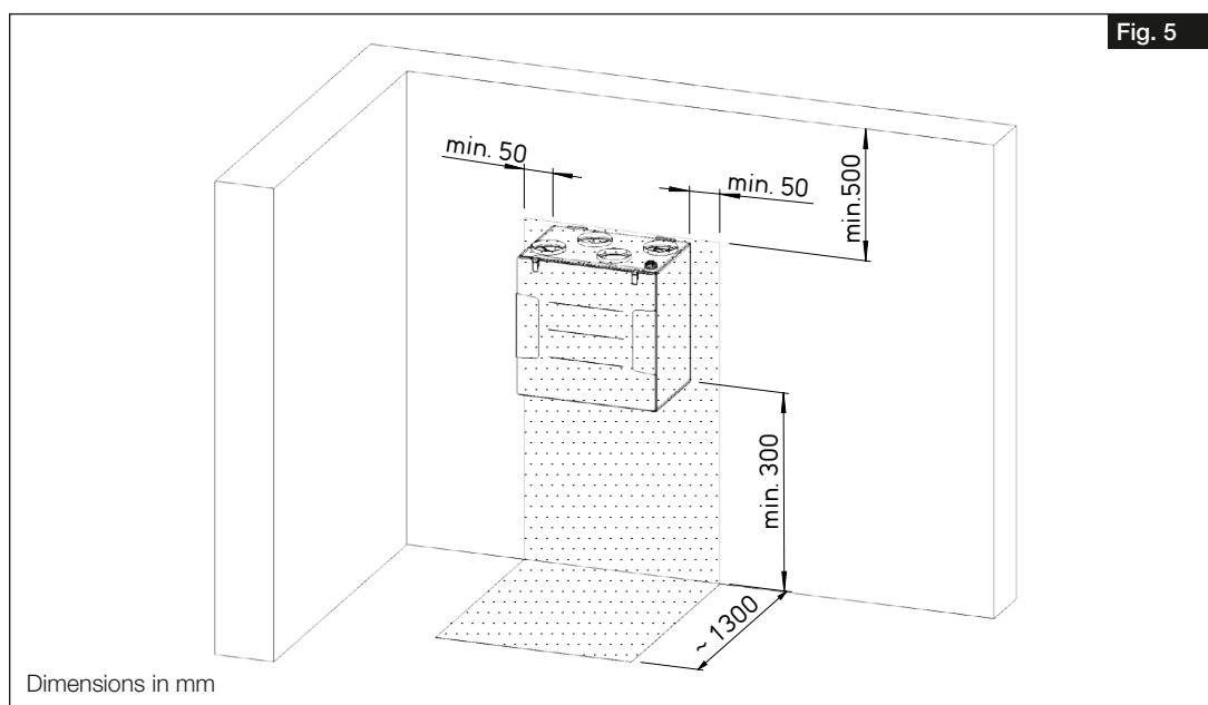
1. The unit may only be installed in frost-free rooms because there is a risk of freezing. The room temperature must not fall below +5 °C.
