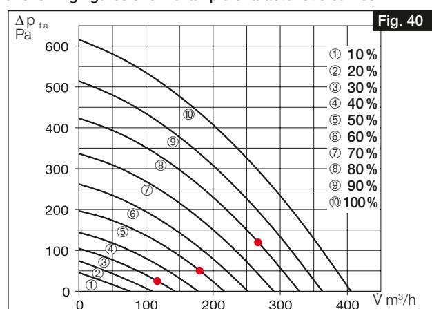
6. If individual measuring points are connected, the system characteristic curve is for supply or extract air (cf. Fig. 41).
