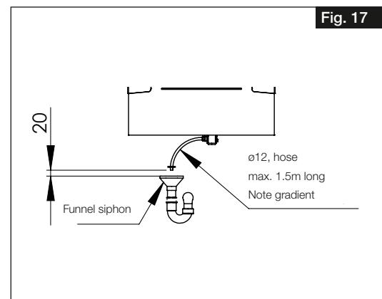
6. Connect condensate hose (length max. 1.5 m) to the building drainage system (see Fig. 18).
