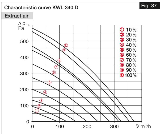
**Determine system characteristic curves for supply and extract air:**
