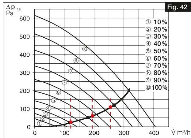
2. The approximate fan powers to be set (in %) can be read from the ventilation profiles at the points of intersection of
